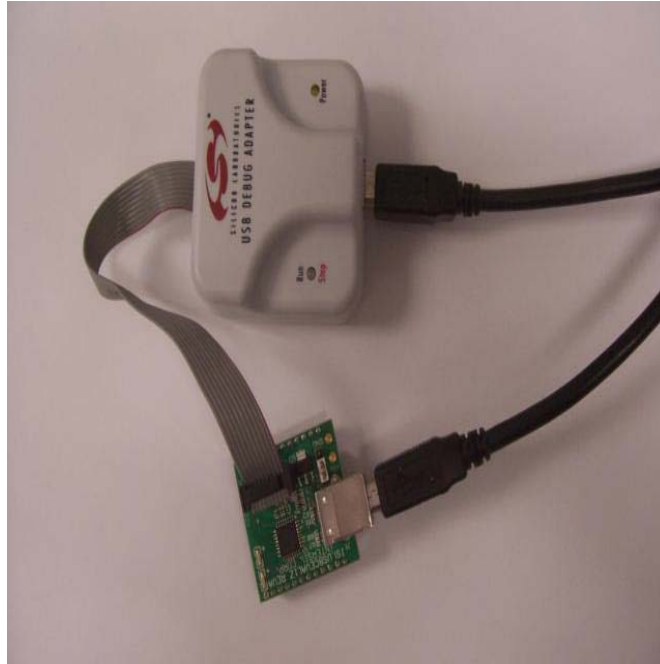
FIGURE 3. SILICON LAB USB DEBUG ADAPTER HOOK UP FOR THE INTERSIL USB DONGLE
